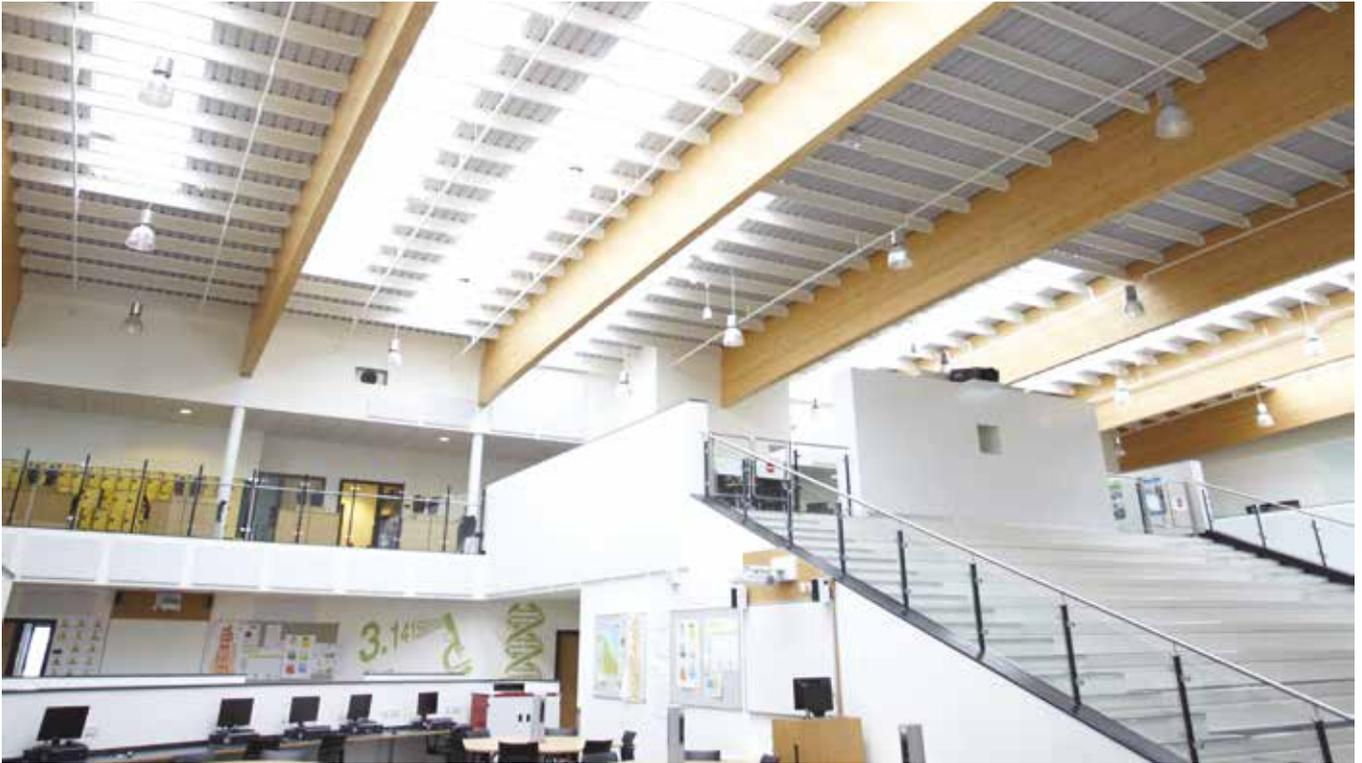
Multivault is an economic, simple to fit barrel vault, which is particularly suitable for large scale cost sensitive projects. The vaults simply lap together to form rooflight runs of unlimited length with spanning capabilities of 1 to 4 metres.
