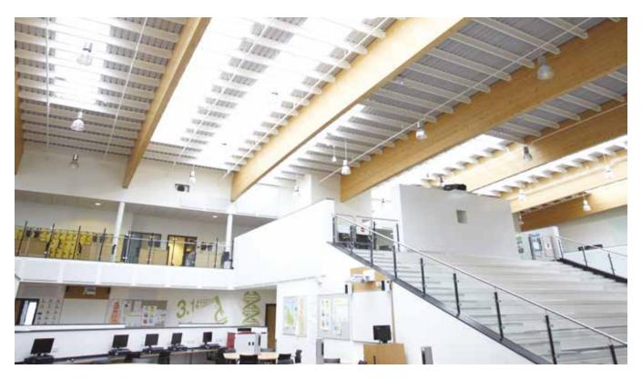
Multivault is an economic, simple to fit barrel vault, which is particularly suitable for large scale cost sensitive projects. The vaults simply lap together to form rooflight runs of unlimited length with spanning capabilities of 1 to 4 metres.
